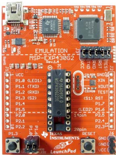
Fotografia 8. Zestaw MSP430 LaunchPad Value Line Development Kit (MSP-EXP430G2)
