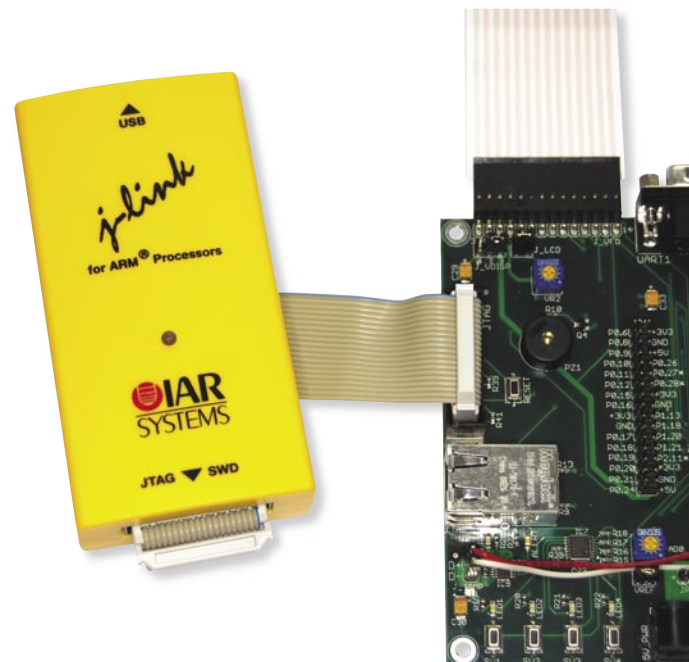
Fot. 2. Debugger/programator JTAG IAR Systems
